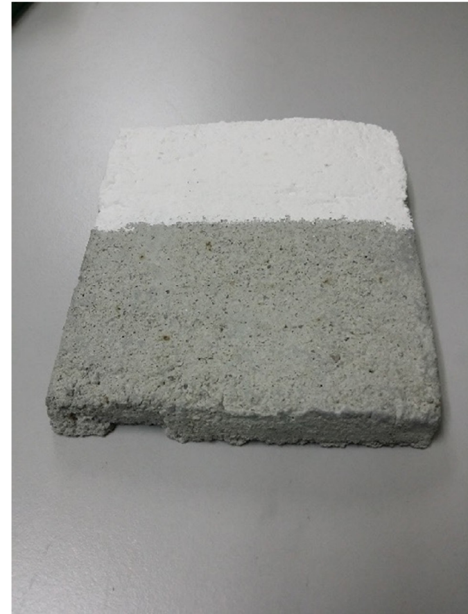
Painted surface does not show colour chang
